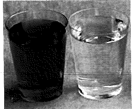
Left: Untreated water distribution system resulting in red water at point of use.
