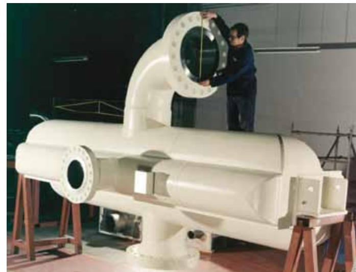
Gas/gas exchanger, 11 MW, 55 bar with 3°C temperature approach. This exchanger was installed in a Joule-Thomson type gas dew pointing system offshore. The close temperature approach allowed a reduction in pressure let down necessary to achieve the low temperature required in the separator, while minimising space and weight.
