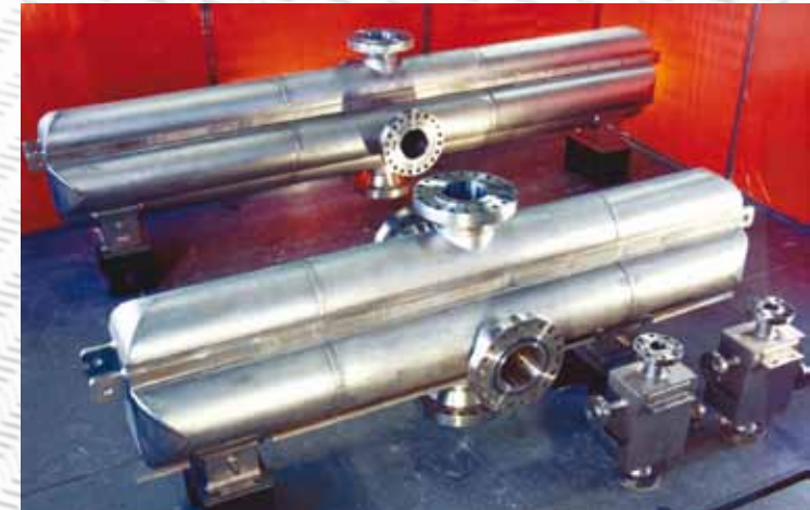
Gas/gas PCHE for J-T dewpoint control
