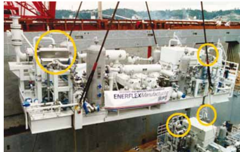
Compact compressor skids each compressing 20 mmscf gas to 175 bar. Photo courtesy of Enerflex Ltd.
