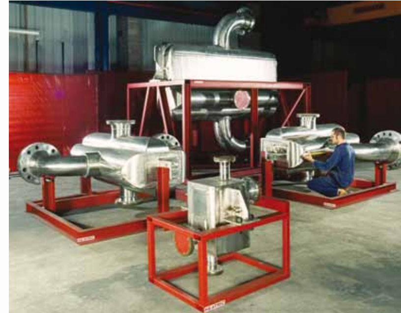
PCHE use on BG Armada saved 3 metres on each of three decks, and enabled single lift installation. The project team estimated GB£10 million (approx. US$15 million) was saved on overall project costs.
