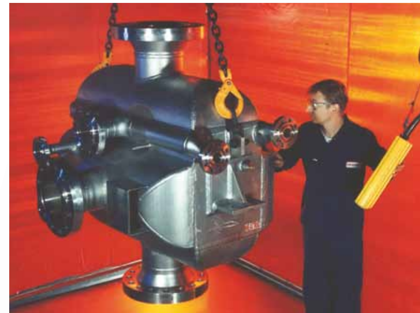
PCHE multi-stream solution for retrofit gas dewpointing in severe space restrictions.
