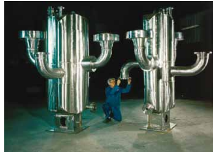
Flexible core orientation and nozzle design can further reduce space requirements. 2 x 11.2 MW gas coolers, 307 bar.
