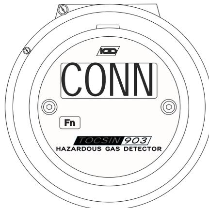
This indicates a communication error between the T903 and detector.
