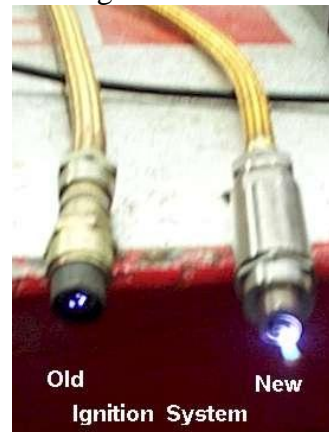
Booster coil (64/51001096) with a Lodge plug (TA-23119). Both old and new are powered by the same 24VDC power supply
