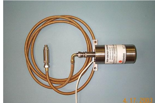
The illustration above shows the igniter plug, adapter and housing.
