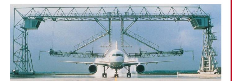
In this application Sigma Eurolock switches are combined with extra long flexible antennae to provide accurate position sensing for an airliner de-icing process. This is just one example from a vast number of diverse applications where the unique characteristics of Sigma switches mean they are the best (and sometimes only) choice.
