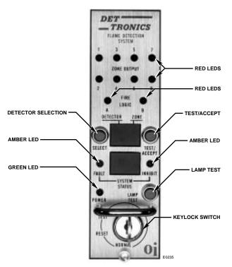
Figure 2—Front Panel of R7404
