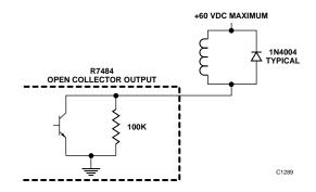
Figure 21—Transient Suppression Device
