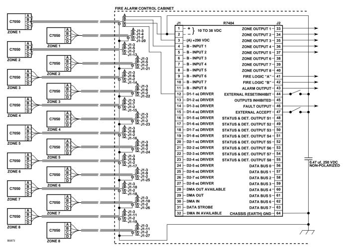
Figure 24—A Typical System – 16 Detectors in 8 Zones
