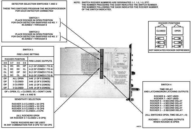
Figure 13—Rocker Switches
