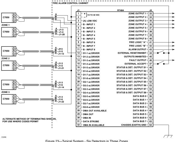
Figure 23—Typical System - Six Detectors in Three Zones
