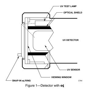
tem. The main loop of the operating program continuously cycles through the Automatic Optical Integrity test, checking each detector and its wiring. At the same time, the microprocessor can be interrupted by any one of several status changes, such as a fault, a "fire" signal from one of the detection zones, or a change in the setting of the keylock switch. In the event of a status change, the microprocessor will take the appropriate action.
