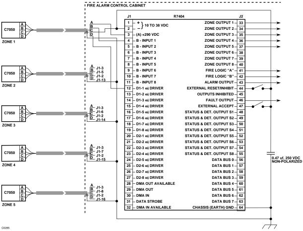
Figure 22—Typical System - Five Detectors in Five Zones
