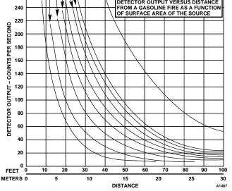
Figure 8—Sensitivity of a Typical Detector to a Gasoline Reference Fire
